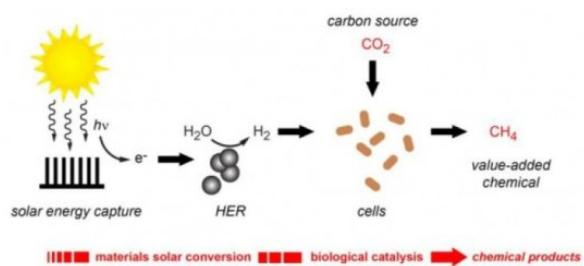
Artificial photosynthesis used to produce renewable molecular hydrogen for synthesizing carbon dioxide into methane.
